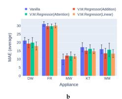
**Figure 11.** Experiment 1: Ablation study to highlight the effect of variational inference on the performance of the model: (a) F1 in category 2: Train and inference on different buildings of UKDALE; (b) MAE category 2: Train and inference on different buildings of UKDALE.
