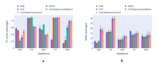
**Figure 17.** Experiment 4: single-target vs multi-target models in category 2, where training happens on UKDALE 1 and inference on UKDALE 2 houses: (a) F1 score in category 2, higher is better; (b) MAE in category 2, lower is better.
