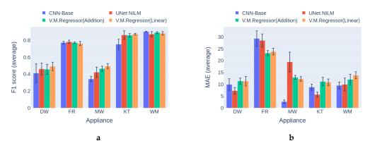
**Figure 12.** Experiment 3: Performance comparison of multi-target models in category 1 where training and inference on happen on UKDALE 1 house: (a) F1 in category 1, higher is better; (b) MAE in category 1, lower is better.
