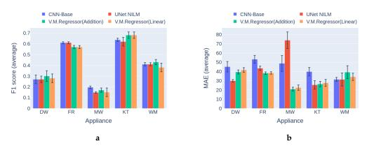
**Figure 15.** Experiment 3: Performance comparison of multi-target models in category 3, where training happens on UKDALE 1 house and inference on REFIT 2 house: (a) F1 in category 3, higher is better; (b) MAE in category 3, lower is better
