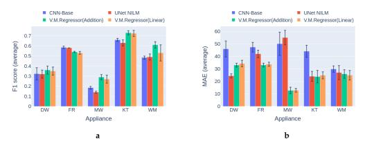
**Figure 14.** Experiment 3: Performance comparison of multi-target models in category 3, where training happens on UKDALE 1 house and inference on REFIT 2 house: (a)F1 in category 3, higher is better; (b) MAE in category 3, lower is better
