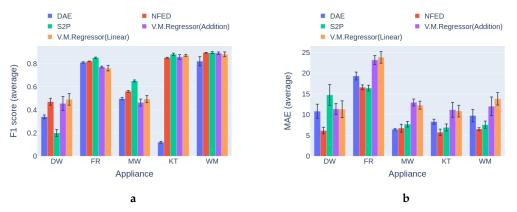
**Figure 16.** Experiment 4: single-target vs multi-target models in category 1, where training and inference on happen on UKDALE 1 house: (a) F1 in category 1, higher is better; (b) MAE in category 1, lower is better
