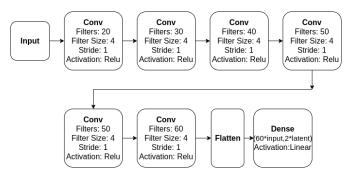
Figure 6. Architecture of ConvEncoder.
