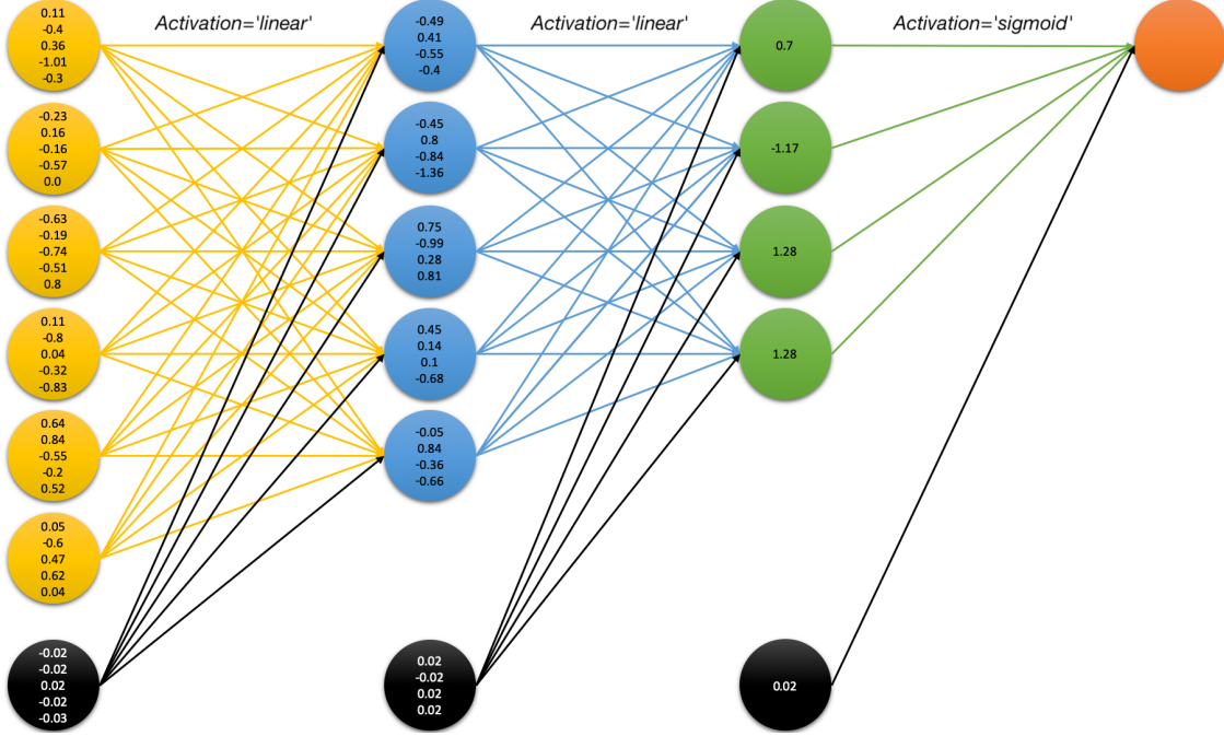
Figure 2: A simple neural network architecture for binary classification
