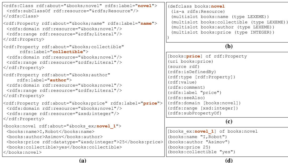
Fig. 11. (a) RDF document excerpt, describing the “novel” class and its properties, as well as an instance of the class (“novel_1”), (b) definition of class “novel” in COOL, (c) transformation of an RDFS property into a COOL object, (d) COOL object, representing the novel instance in (a)
