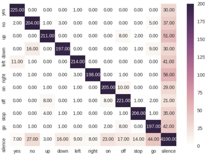
Fig. 3. Confusion matrix with results of the proposed neural network recognizing 10 different speech commands.
