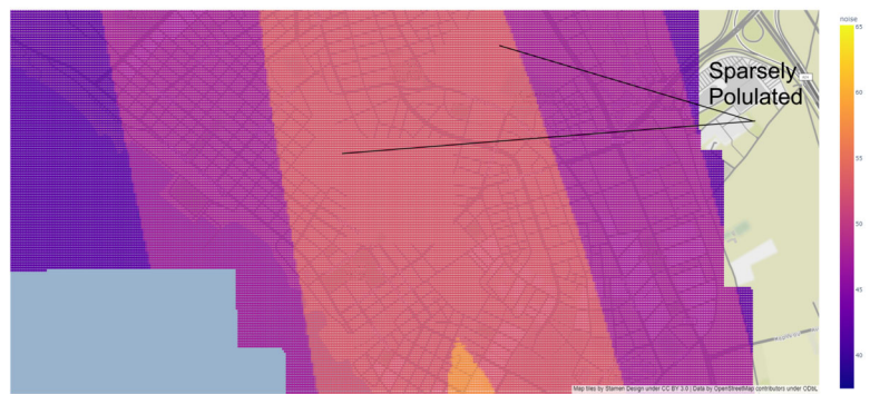
Figure 8 Average nightly aviation noise in Kalamaria. This is the reconstructed heatmap that corresponds solely to the aviation noise. The two sparsely populated areas are marked accordingly. Lighter colors indicate more noise, while darker, less noise
