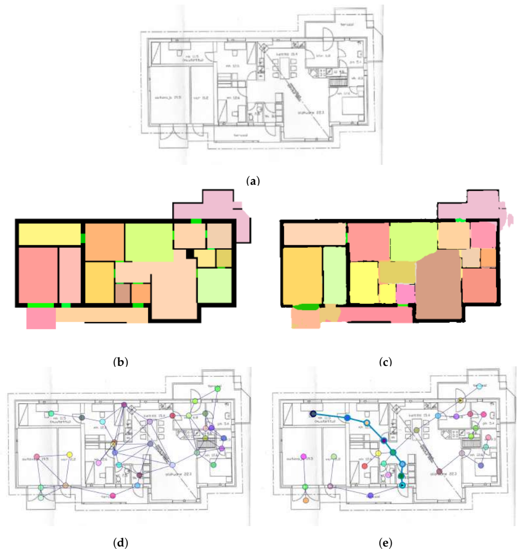
Figure 11. Floor plan 8: (a) Original image. (b) Panoptic label. (c) Panoptic prediction. (d) Graph. (e) Final graph and path.
