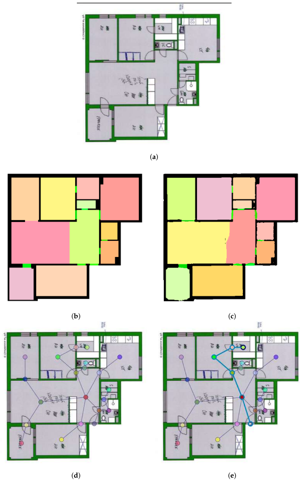
Figure 9. Floorplan 6: (a) Original image. (b) Panoptic label. (c) Panoptic prediction. (d) Graph. (e) Final graph and path. Highlighted is the returned path
