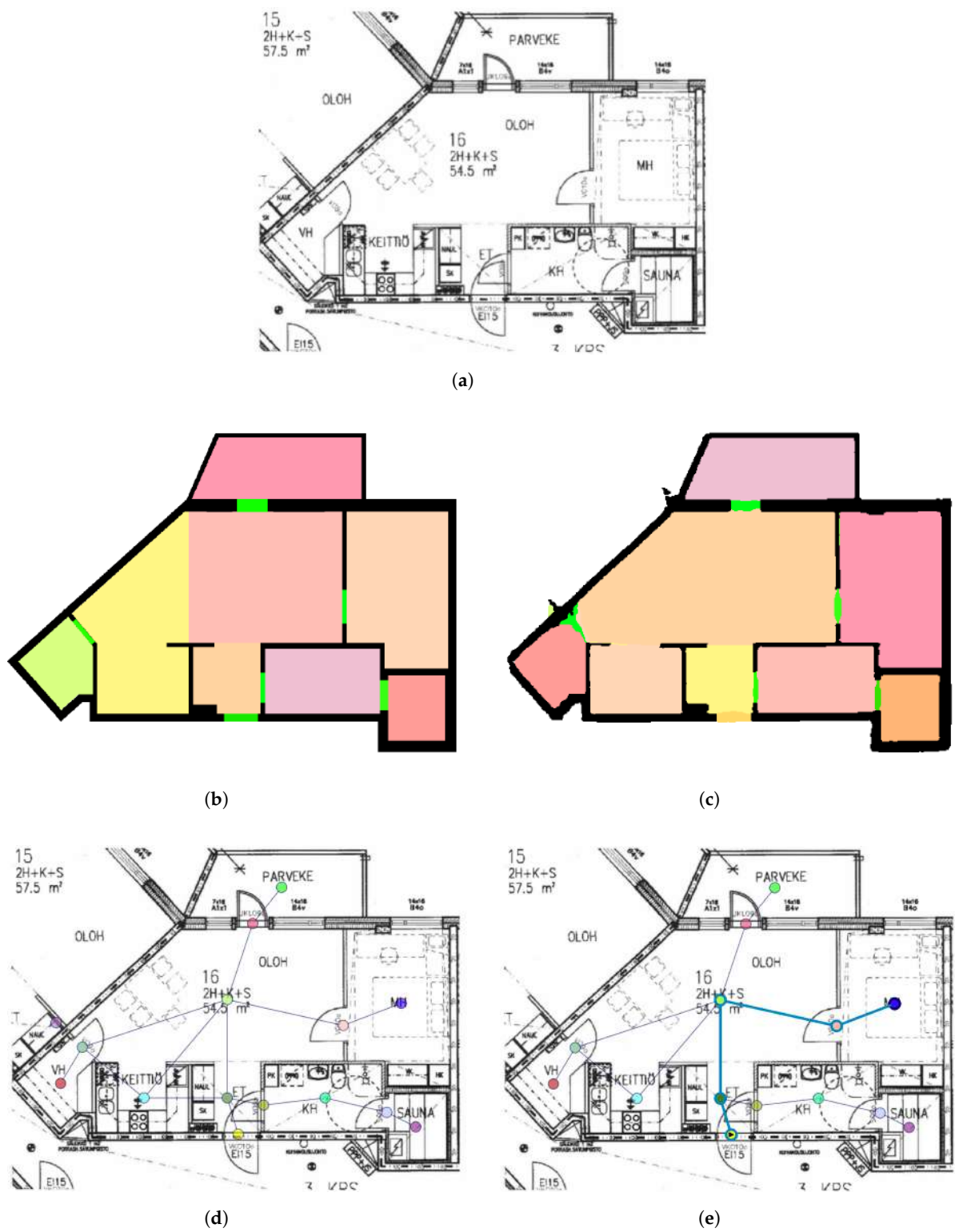
Figure 8. Floor plan 5: (a) Original image. (b) Panoptic label. (c) Panoptic prediction. (d) Graph. (e) Final graph and path.
