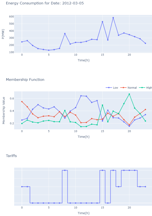
Figure 2: Energy Consumption, Membership Function, and FCM Tariffs in Low Carbon London dataset
